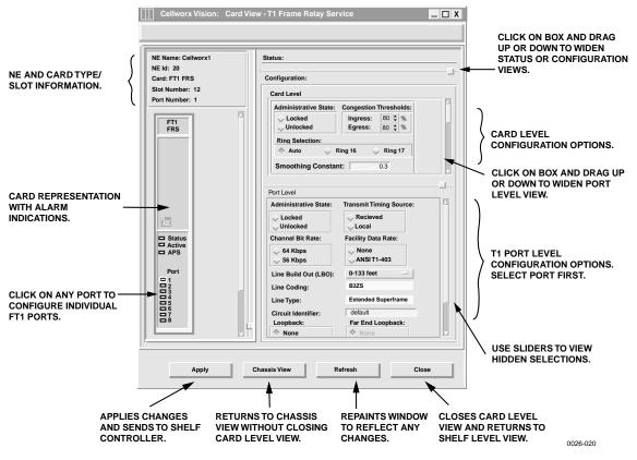
Figure 785-1. FT1 FRS Card Configuration Window
